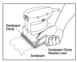
FIGURE 3. INSTALLING THE SANDPAPER
